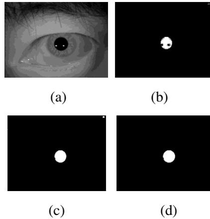
Fig 4: Steps for the detection of the internal contour of the iris:(a) eye image; (b) binary image  $I_{\text{bin}}$  (c) closing of the binary image  $I_{\text{bin}}$ ; (d) opening of the binary image  $I_{\text{bin}}$ .
