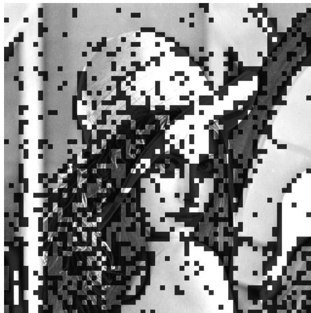
Fig. (1) Domain blocks of size 8x8 that are used for fractal encoding of Lena image are shown in black.
