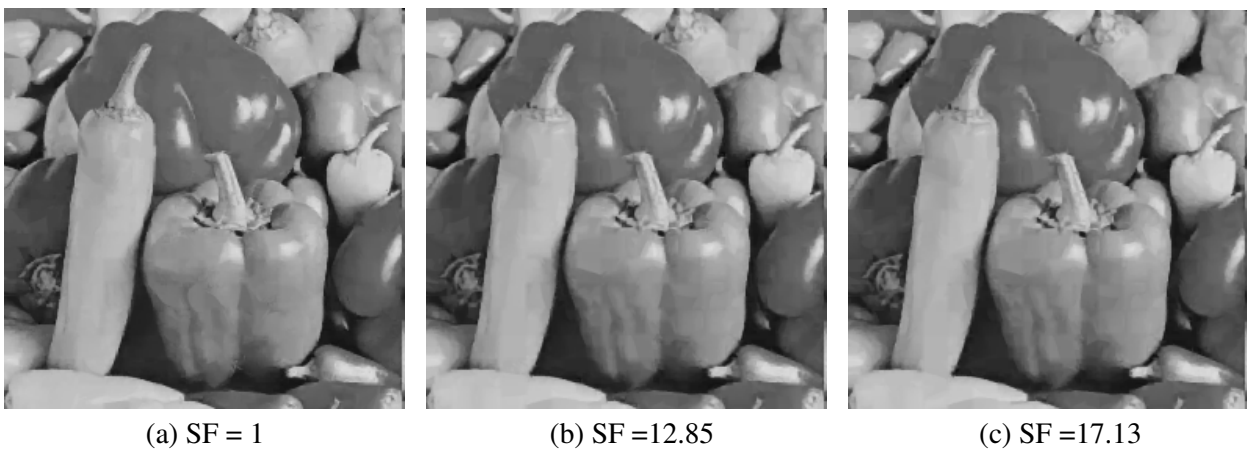
Fig. (6): Reconstructed image Peppers by full search (a): PSNR=31.91, MSSIM= 0.8931 and by the proposed method (b): PSNR= 31.13 dB, MSSIM = 0.8842 and (c): PSNR=30.90 dB, MSSIM=0.8813.
