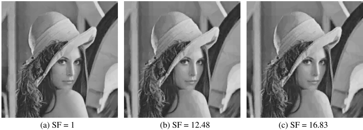
Fig. (5): Reconstructed image Lena by full search (a): PSNR = 30.92 dB, MSSIM = 0.8909 and by the proposed method (b): PSNR = 30.16 dB, MSSIM = 0.8836 and (c): PSNR = 29.88 dB, MSSIM = 0.8807.
